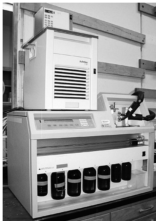
Figure 9. Automated oligosaccharide synthesizer developed by Seeberger and co-workers (adapted from: Chem. Eur. J. 2005 , 11 , 3194–3206).
